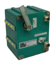
Due to the low moment of inertia of the motor discs nevertheless quick response times can be gained. In case of voltage loss a return spring ensures setting back to zero position. Optionally the actuator is available without return spring. A contactless feedback system is integrated onto the governors output shaft offering an electrical position signal to any external control unit.
